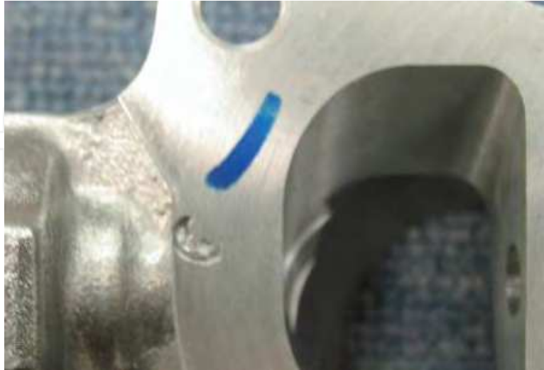
Fig. 9. Photograph of blow hole
