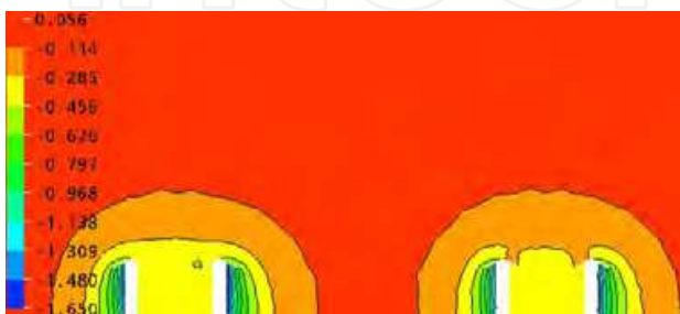
(e) Wind pressure coefficient of center profile when S = 2D
