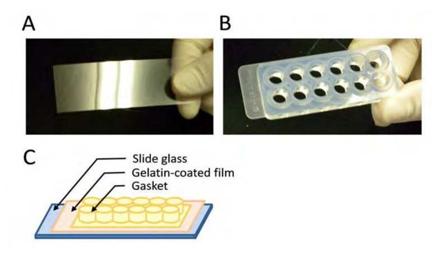
A: gelatin-coated film, B: gasket, C: illustration of the assembled detection system
