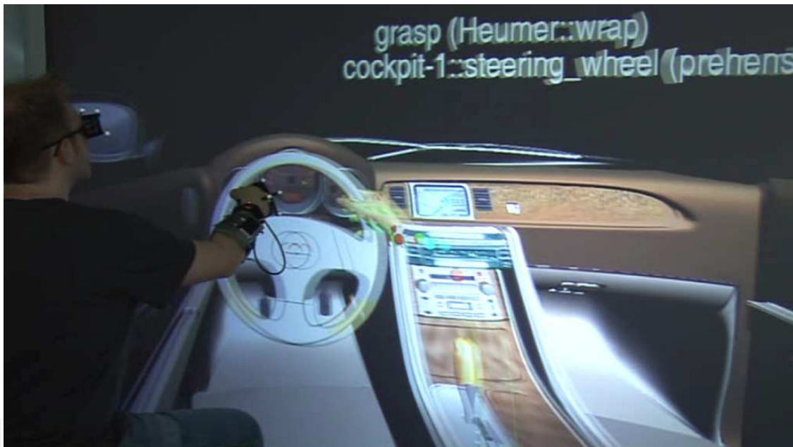
Fig. 9. Automatic recognition of basic interactions while manipulating the control actuators of a virtual car interior.
