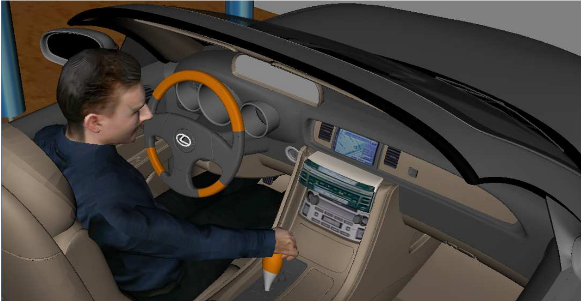
Fig. 12. Control actuators contained in the virtual prototype of a car cockpit.
