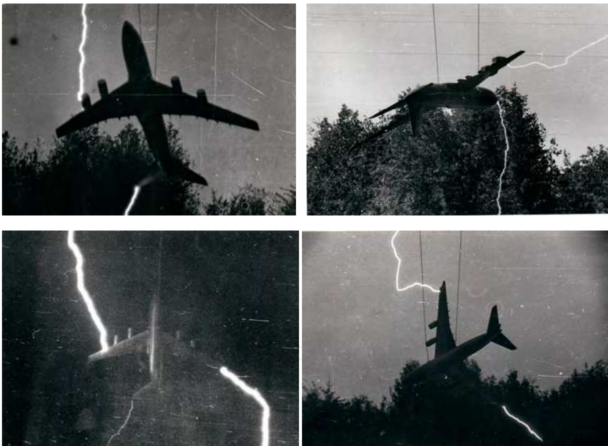
Fig. 19. Laboratory testing of lightning strikes to an aircraft model.
