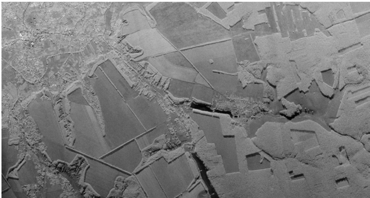
Fig. 17. An example of a 7-look SAR image obtained with the X-band SAR system.
