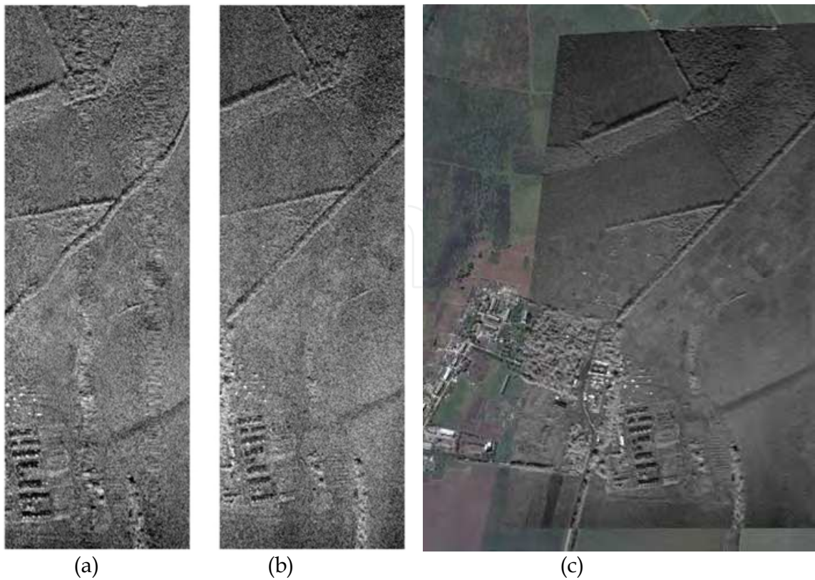
Fig. 13. Illustration of the geometric correction: (a) the 3-look SAR image built by using the clutter-lock technique, (b) the 3-look SAR image formed by using the built-in geometric correction, and (c) the 45-look SAR image formed by using the built-in geometric correction is imposed on the Google Maps image of the scene.
