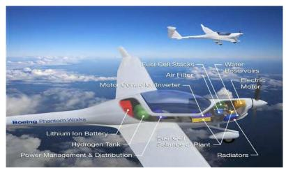
Fig. 33. Boeing PEM Fuel Cell Powered Electric Aircraft [36].
