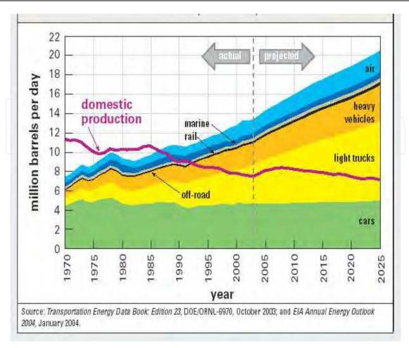
Fig. 4. Fuel consumption in U.S by transport vehicles [2].
