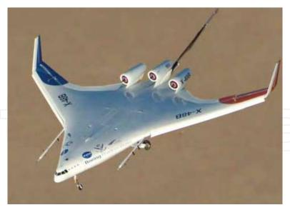
Fig. 23. Boeing/NASA X-48B BWB technology demonstrator aircraft [23].
