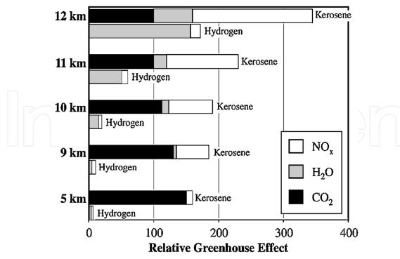
Fig. 36. Relative emissions from Jet-kerosene and Hydrogen at various altitudes [39].
