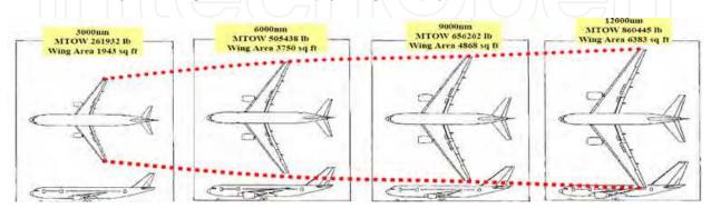
Fig. 32. Aircraft designs, with fixed fuselage, 250 passengers and  $C_{L}$ , for different ranges of operation [30, 31].
