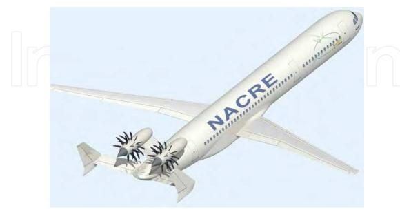
Fig. 21. Open-Rotor version of pro-active Green Aircraft in NACRE study [17].
