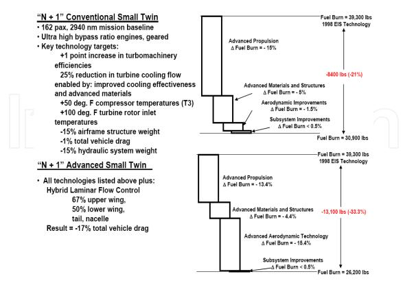
Fig. 25. Reduction in fuel burn for N+1 generation aircraft relative to baseline B737/CFM56 using advanced technologies [26].
