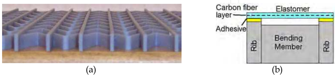
Fig. 13. EMC-structure bonding method – (a) honeycomb core; (b) single cell diagram.
