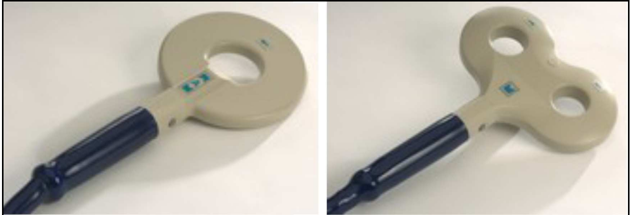
Fig. 2. The two most common TMS coils: (left) the circular coil and (right) the 8-shaped coil.
