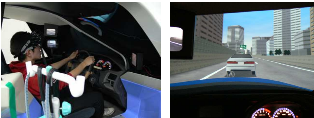
Fig. 18. Experiment with driving simulator (driver follows the proceeding vehicle with and without ACC)
