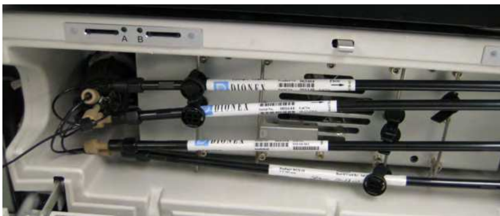
Fig. 13. HPLC column compartment equipped with a 6-port column switching valve, for screening of up to six different columns for pH-IEC without the need to change buffers or columns.
