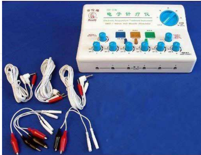
Fig. 5. An electric apparatus for electroacupuncture stimulation
