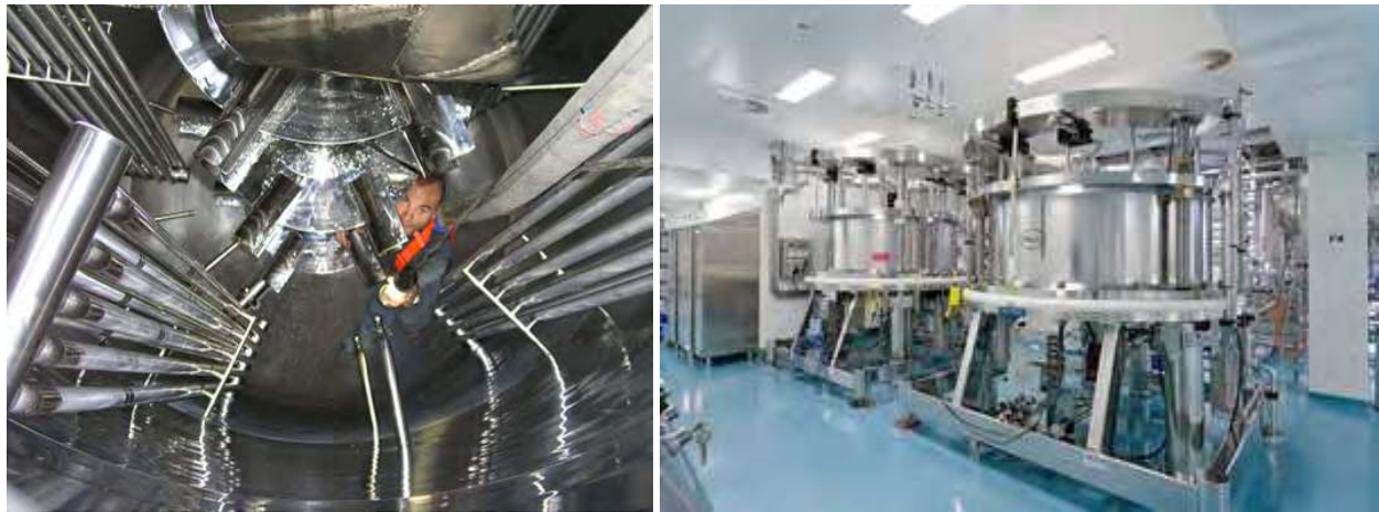
Fig. 1. Left side: photograph of a 15m 3 state of the art sterile containment for high cell density fermentations. LONZA has built and operates such high performance equipment up to the 75m 3 for a range of organisms including methylotrophic yeasts such as Pichia pastoris . The flow breakers are designed as cooling elements needed to remove metabolic heat. The stirrers are concave Rushton impellers which, in combination with specially designed dip pipes (not shown), allow optimal mixing. In most cases the stirrer configuration is completed by the use of a top radially downward pumping marine impeller. Right: Two chromatography columns for the purification of injectable therapeutic proteins with a diameter of 2 meters to demonstrate size and complexity of down stream processing (Copyright@Lonza).
