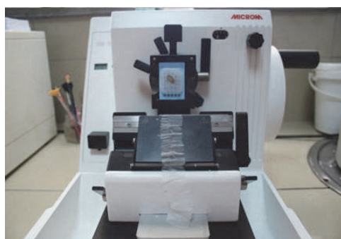
(e) Execution of histological sections with a rotary microtome
