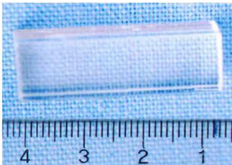
Fig. 4.1. Image of the unprocessed cleavage microchip along the (101) planes directly obtained from the as-grown crystal
