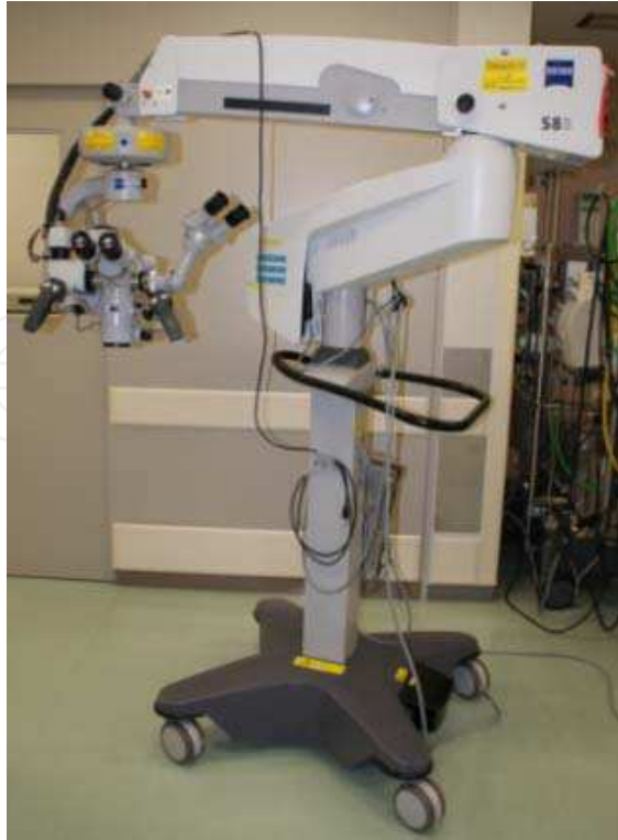
Fig. 4. The surgical microscope used for microvascular hepatic artery reconstruction (Carl Zeiss, OPMI VARIO S88). This microscope has a foot pedal. The surgeon can adjust the microscope using this foot pedal without interrupting the procedure
