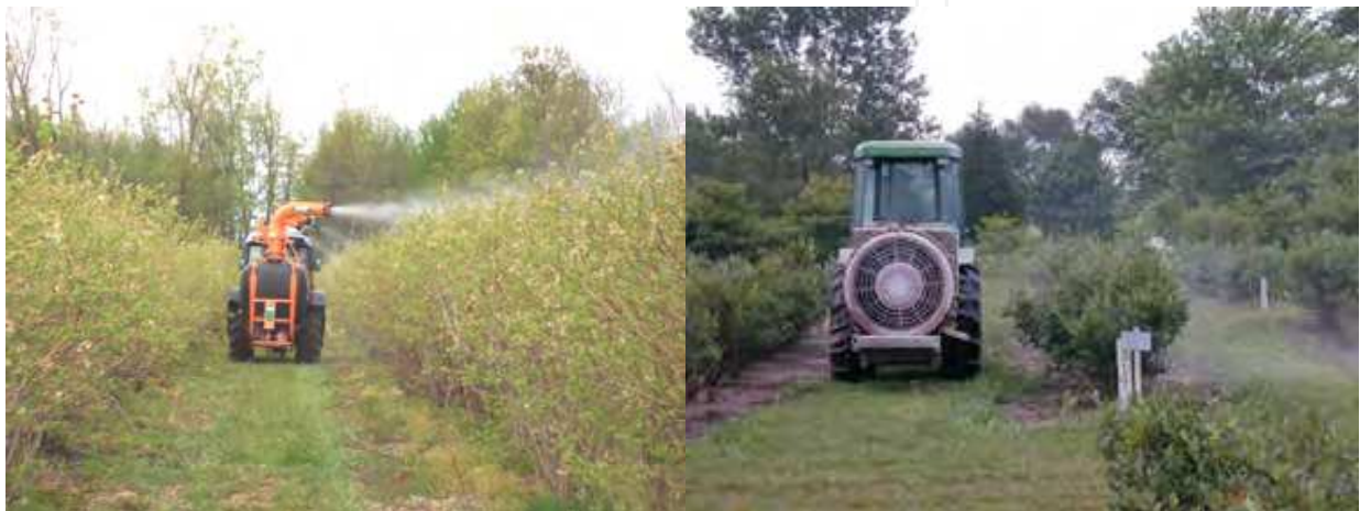
Fig. 5. Air assisted sprayers: right, a cannon sprayer; left, conventional air-blast sprayer.
