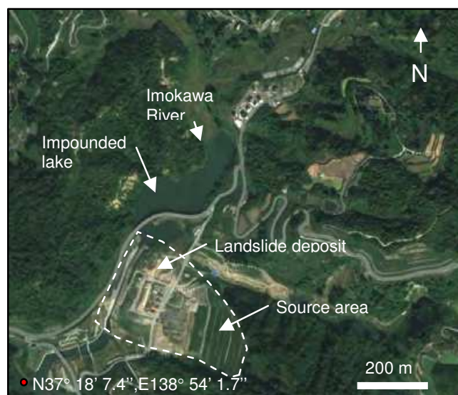
Fig. 3. Higashi Takezawa landslide dam and the dammed lake (Satellite imagery from Google Map)
