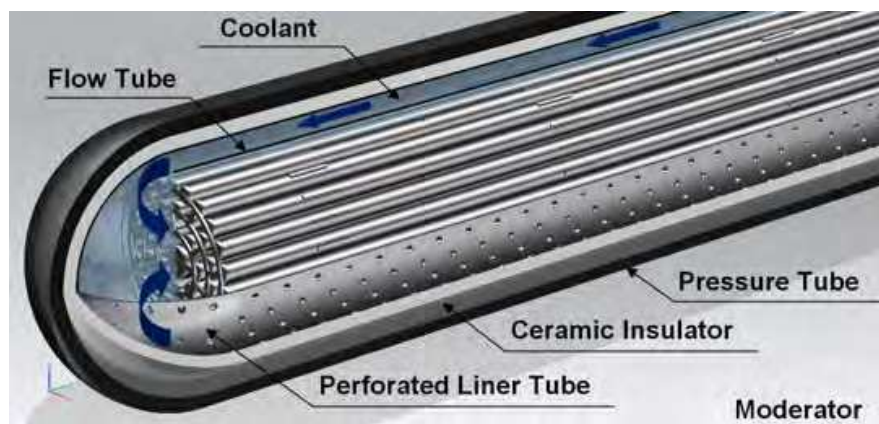
Fig. 8. Re-entrant fuel channel with ceramic insulator.
