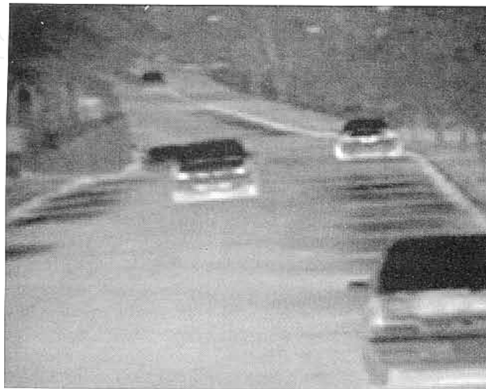
Fig. 25. This picture was taken at the night (around midnight) and it clearly shows where automobiles were parked during the daytime. This image demonstrates the high sensitivity of the 640×486 long-wavelength QWIP staring array (Guapala et al., 1998).
