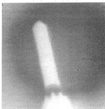
Fig. 32. Image of a Delta-II launch vehicle taken with the long-wavelength QWIP RADIANCE during the launch (Guapala et al., 2001).
