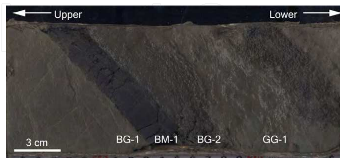
Fig. 18. Black material zone distributed at about 1194 m depth in the TCDP Hole B cores.
