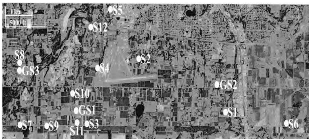
Fig. 1. Aerial map of the sampling area located in the Lower Fraser Valley region of British Columbia, Canada. "S" and "GS" indicate surface water and groundwater sampling sites, respectively. The map was generated using Google Maps
