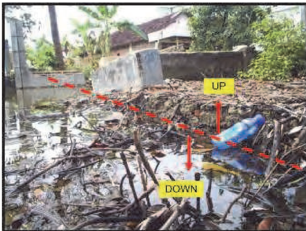
Fig. 20. The pattern of fractures trending NE -SW in the Village Renokenongo. A section of land on the right hand side of the picture is uplifted (east side) while the left is the downthrown block (west side). Note: The mineral water bottle is used as a comparison to indicate the amount of displacement (~20cm). In contrast to Degushi et al., 2007b pseudo anomaly interpretation, the above photo taken 2 months after the eruption suggests displacement due to fault movement. Movement due to subsidence was unlikely as it was minimal at the early stages of the eruption.
