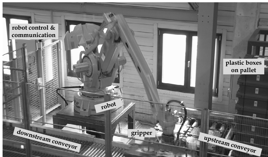
Fig. 9. Industrial application of a robotic system for depalletizing plastic boxes: result of the ontological configuration [source: author's illustration]
