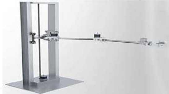
Fig. 6. SolidWorks rendered design of the robotic arm
