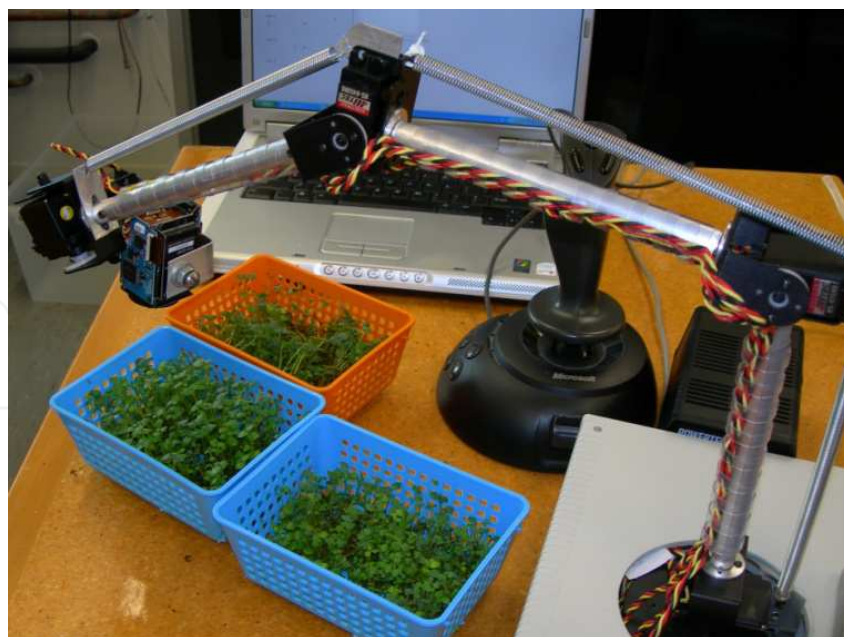
Fig. 3. The completed robotic arm with camera, joystick and plant trays
