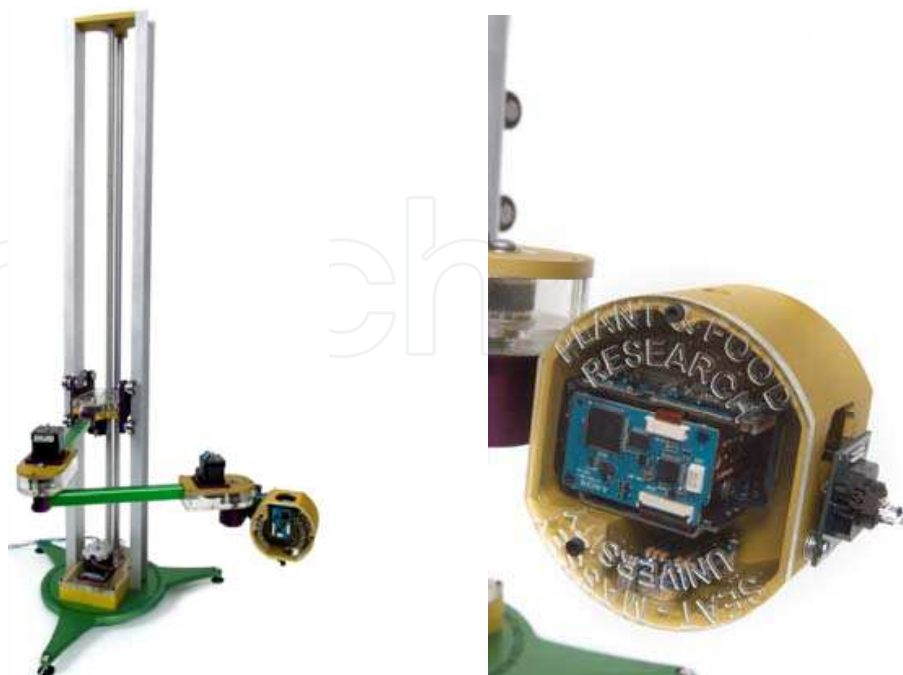
Fig. 8. (a) Completed robotic arm using stepper motors (b) Camera housing and RGB colour Sensors
