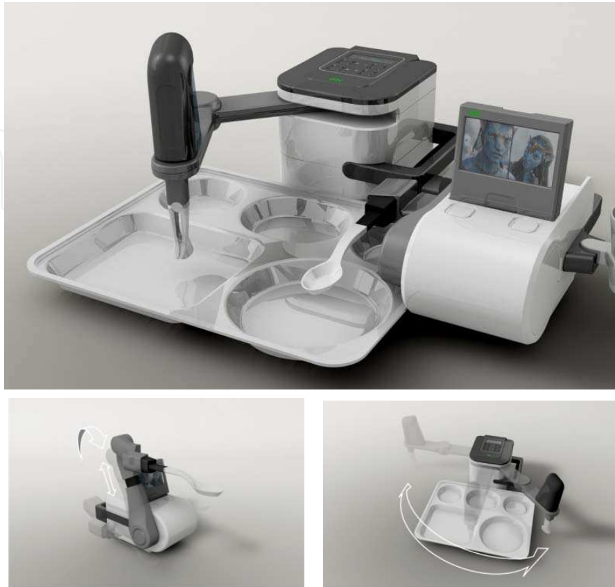
Fig. 9. The design of a novel feeding robot for Korean food. A spoon-arm (lower left-hand-side figure) for transferring food and a grab-arm (lower right-hand-side figure) for picking up and releasing food
