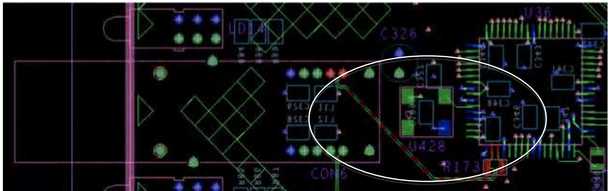
Fig. 16. Unrouted differential lines.
