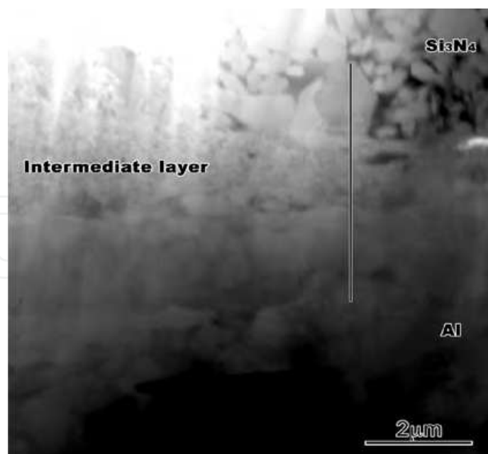
Fig. 7. A STEM image of the interface of Al/Si 3 N 4 clad. EDS line profile shown in Figure 8 was measured along the black line in this figure.
