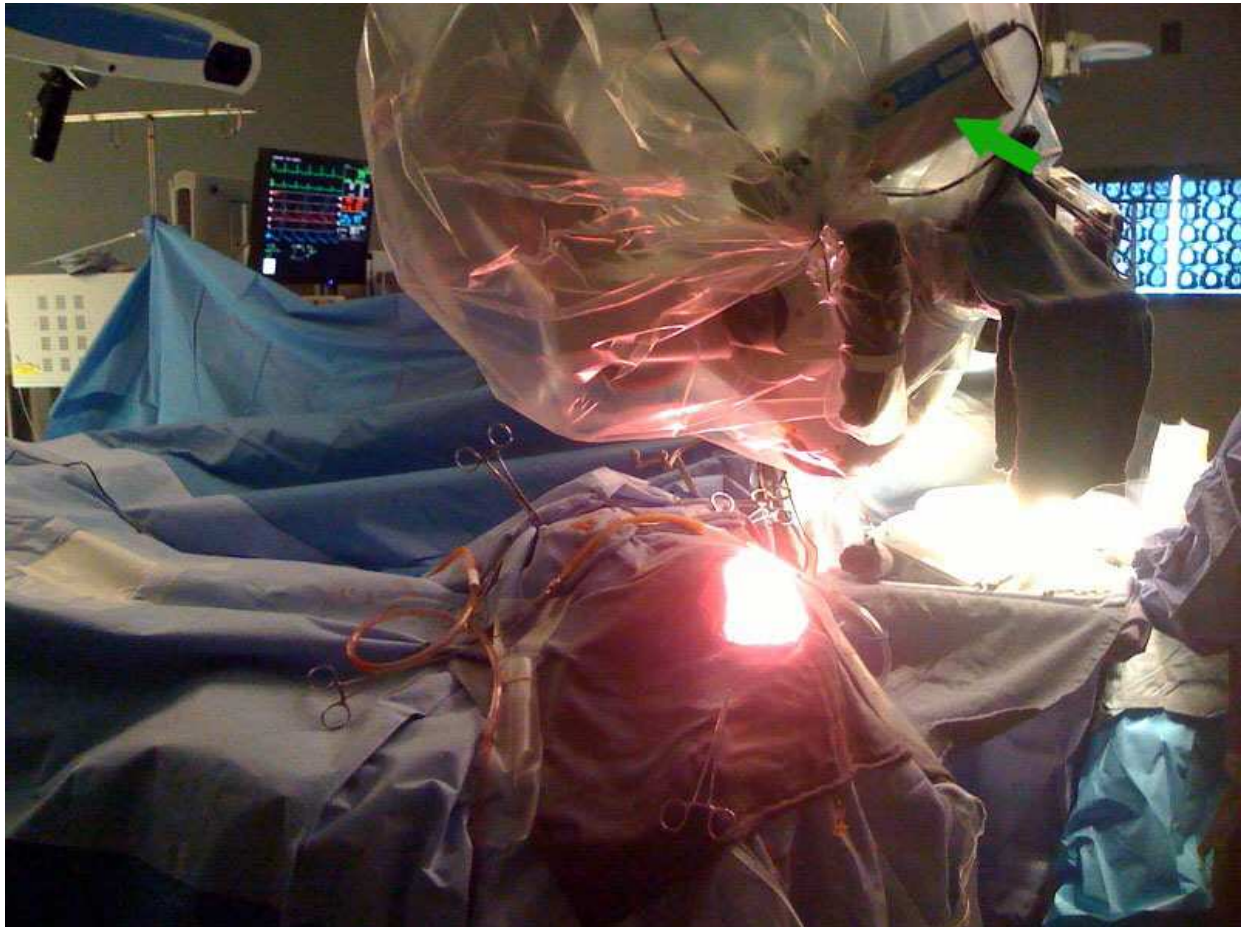
Fig. 3. Intraoperative photograph showing CCD camera mounted on operating microscope. The cortex is illuminated with white light, and the reflected light is filtered at a particular wavelength of interest. Images are captured by a very sensitive CCD camera (shown with green arrow), and reflectance changes between rest and stimulation are measured. These changes correspond to evolving aspects of the hemodynamic response generated as a consequence of underlying cortical activity.
