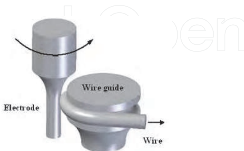
Fig. 4.2. Schematic of tool-electrode dressing by WEDG
