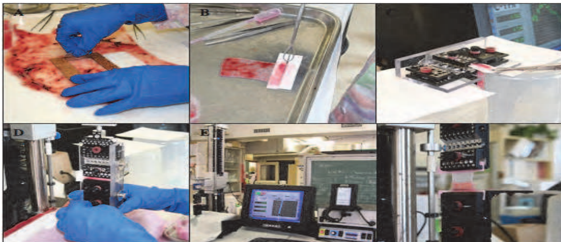
Fig. 3. Peel testing procedures. Tissue samples are cut out from FM kept moist and laid flat and kept moist (A). Stiff filter paper stints assist in holding and mounting the partially manually peeled amnion and choriodecidua by maintaining shape (B). Membrane piece mounted on custom clamps which are maintained in fixed position by a plexiglass mount support to assist sample loading (C). Sample loaded clamps with supporting Plexiglas mount as a single unit attached to the peel testing device (D). The peel tester with the FM piece loaded and the plexiglass mount support removed before beginning the test (E). FM components, amnion and choriodecidua, being peeled apart between the clamp jaws (F).
