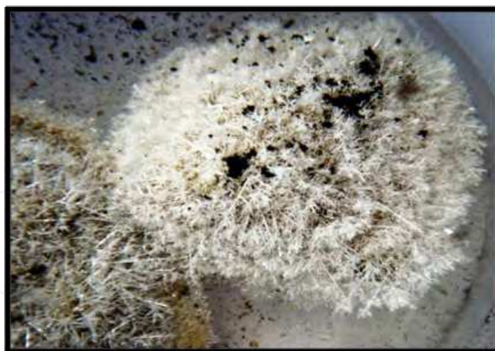
Fig. 14. Another silver dendritic growth with needle-like formation. The black spots on top were holes left by the bubbles ejection.
