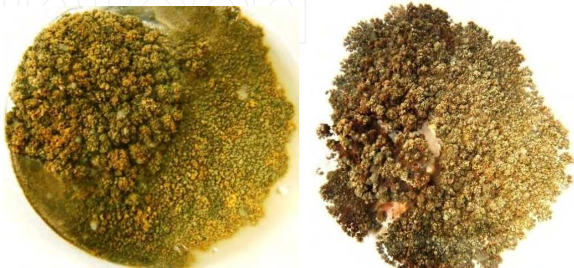
Fig. 15. Two silver deposits, after a month, on Mn pieces located at the center of the formation.
