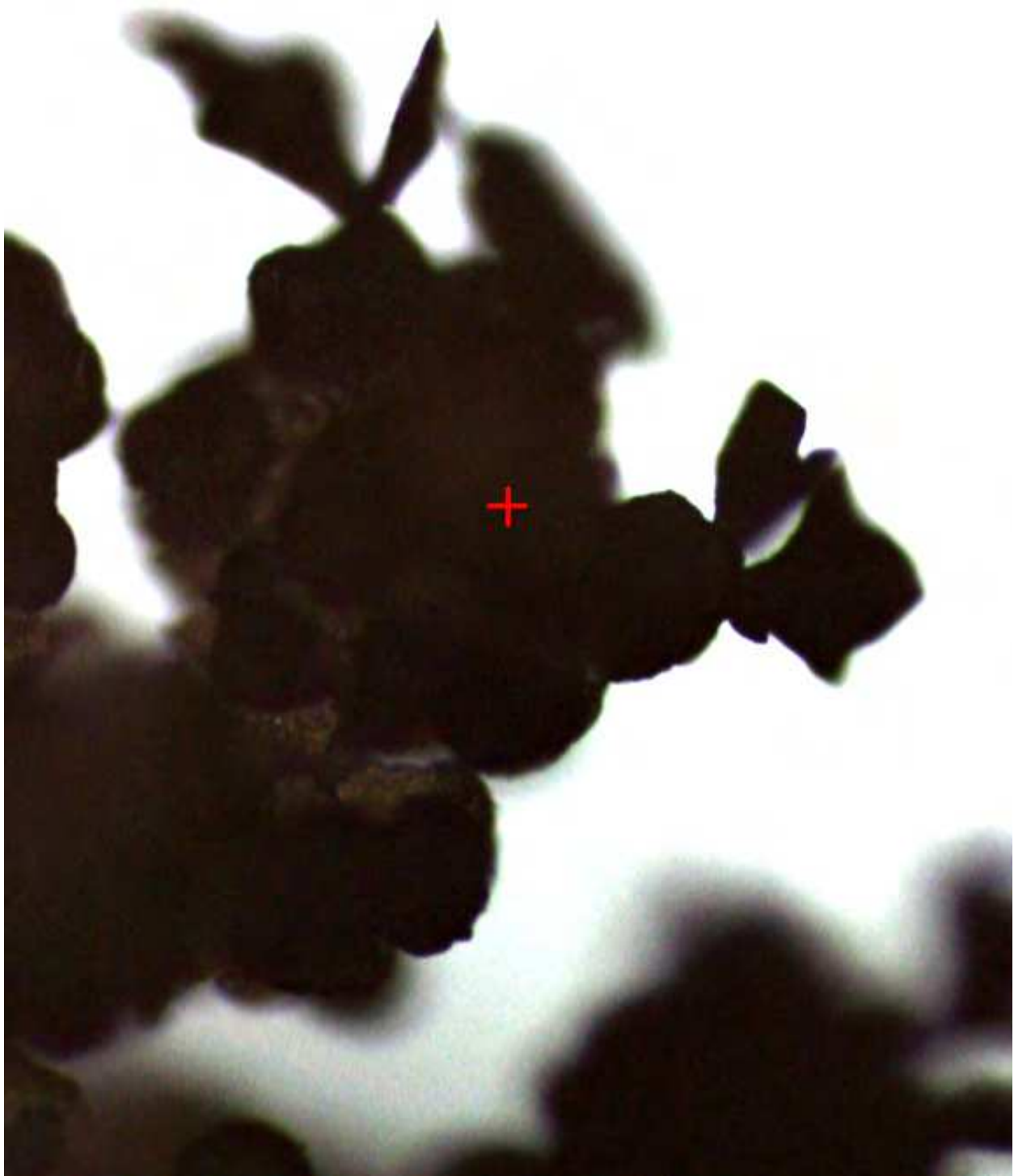
Fig. 10. Image from a lead deposition in an edge of a manganese plate with a semi-dendritic column constituted by grain nucleations and leaves-like forms on top.
