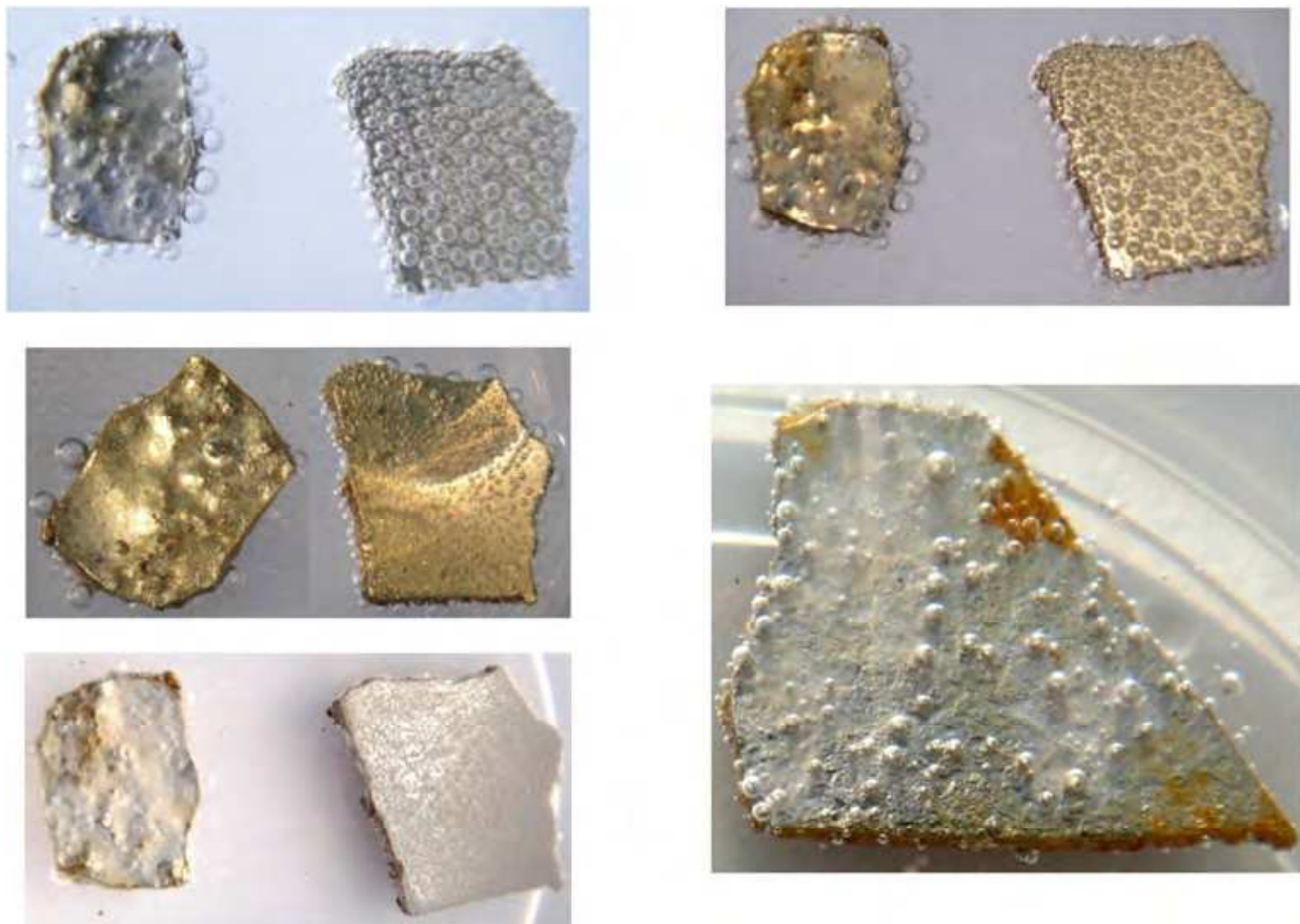
Fig. 18. Aluminum deposits on manganese at different times in the process. The white metallic finishing remained unchanged with exposition to air.
