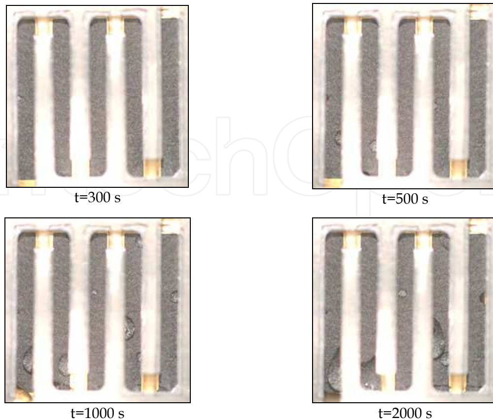
Fig. 6. Visualization images of liquid water behavior on the cathode GDL at 0.16 \text{ A/cm}^2
