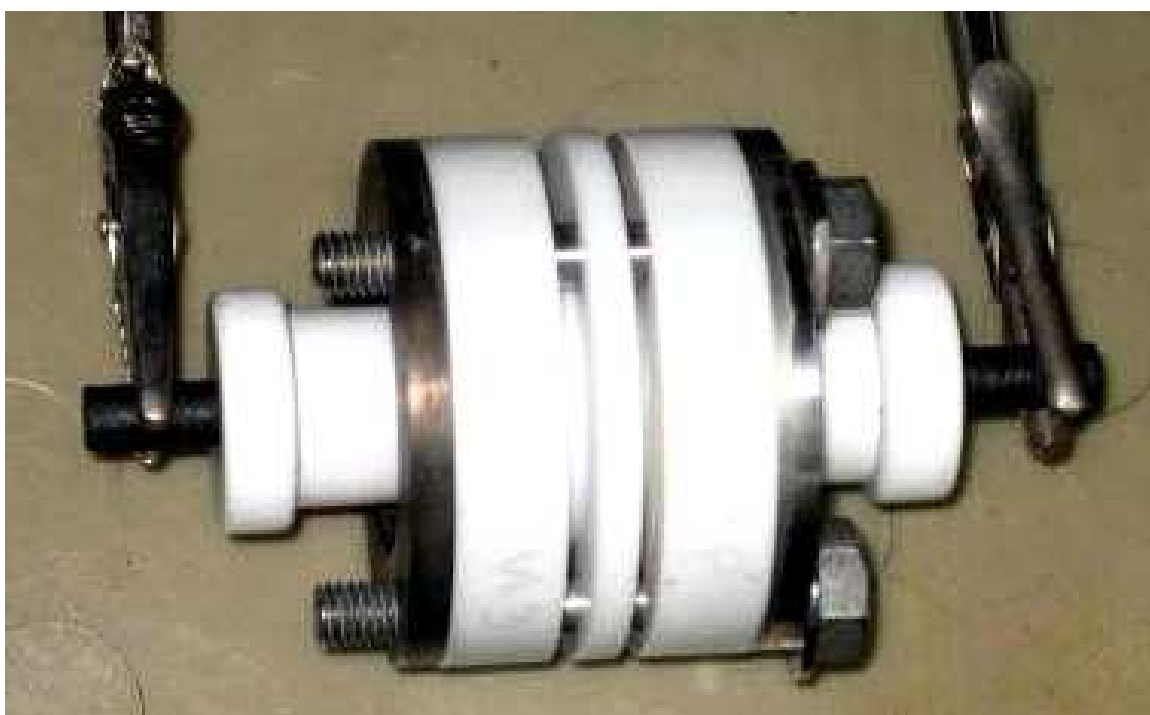
Fig. 2.b Photograph of the electrochemical cell
