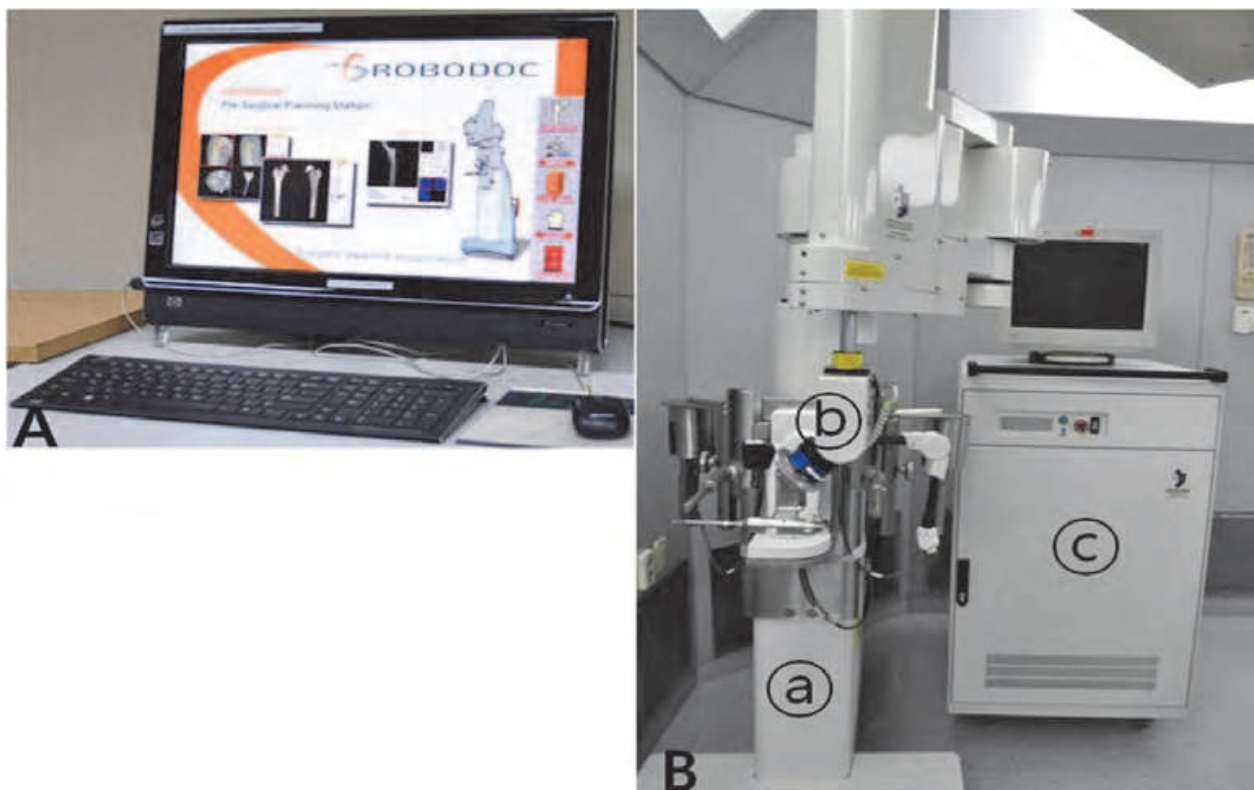
Fig. 9. ROBODOC® system (Integrated Surgical Systems, Davis, CA) is composed of two primary components. (A) CT-based preoperative planning using ORTHODOC, and (B) Robot-assisted surgery using the ROBODOC surgical assistant (a = robot base, b = robot arm, c = the control computer)
