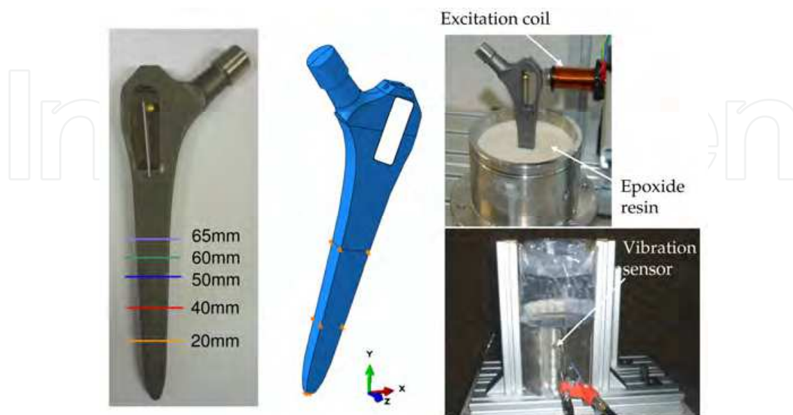
Fig. 14. Left: Prototype of a femoral component with the embedding heights tested in a cylindrical setup with epoxide resin. Middle: Model of the femoral component for finite-element analysis exemplarily with an embedded height of 65 mm. Right: Experimental setup with embedded hip stem and the applied water reservoir with external vibration sensor.
