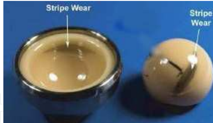
Fig. 11. A ceramic head and acetabular liner from a patient with "squeaking" hip with evidence of impingement and "stripe wear".
