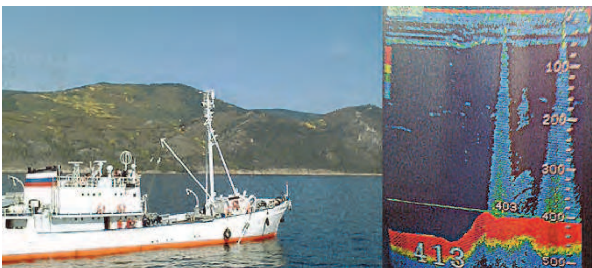
Fig. 23. Sampling gas hydrates, Lake Baikal, 2010. The image on the right is a screen shot of the on-board echosounder (EM400), showing the gas seepage from under-ground gas hydrates on a slight ridge on the lake floor (depth: 403 m below the central seep plume)
