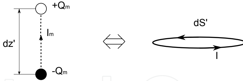
Fig. 7. Magnetic dipole and electrical current loop
