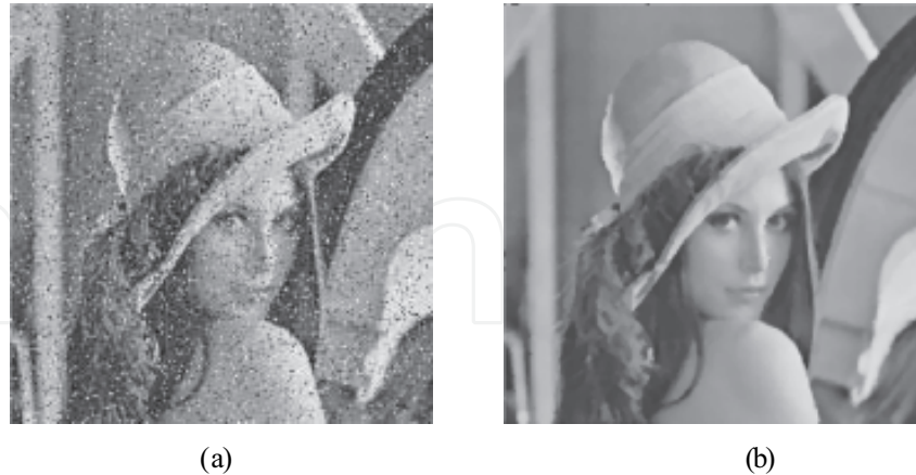
Fig. 42. Simulation results of a 2-D RMF application. (a) The noisy “Lena” image corrupted by 9% of impulsive noise. (b) The “Lena” image processed by the 3 \times 3 RMF.
