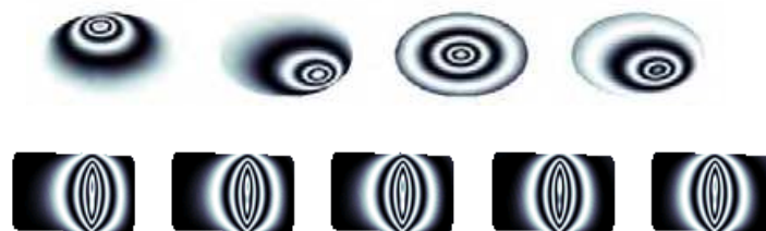
Fig. 8. Examples of interferograms of the influence functions generated by the actuators for a round membrane DM (top) and for a rectangular membrane DM (bottom).
