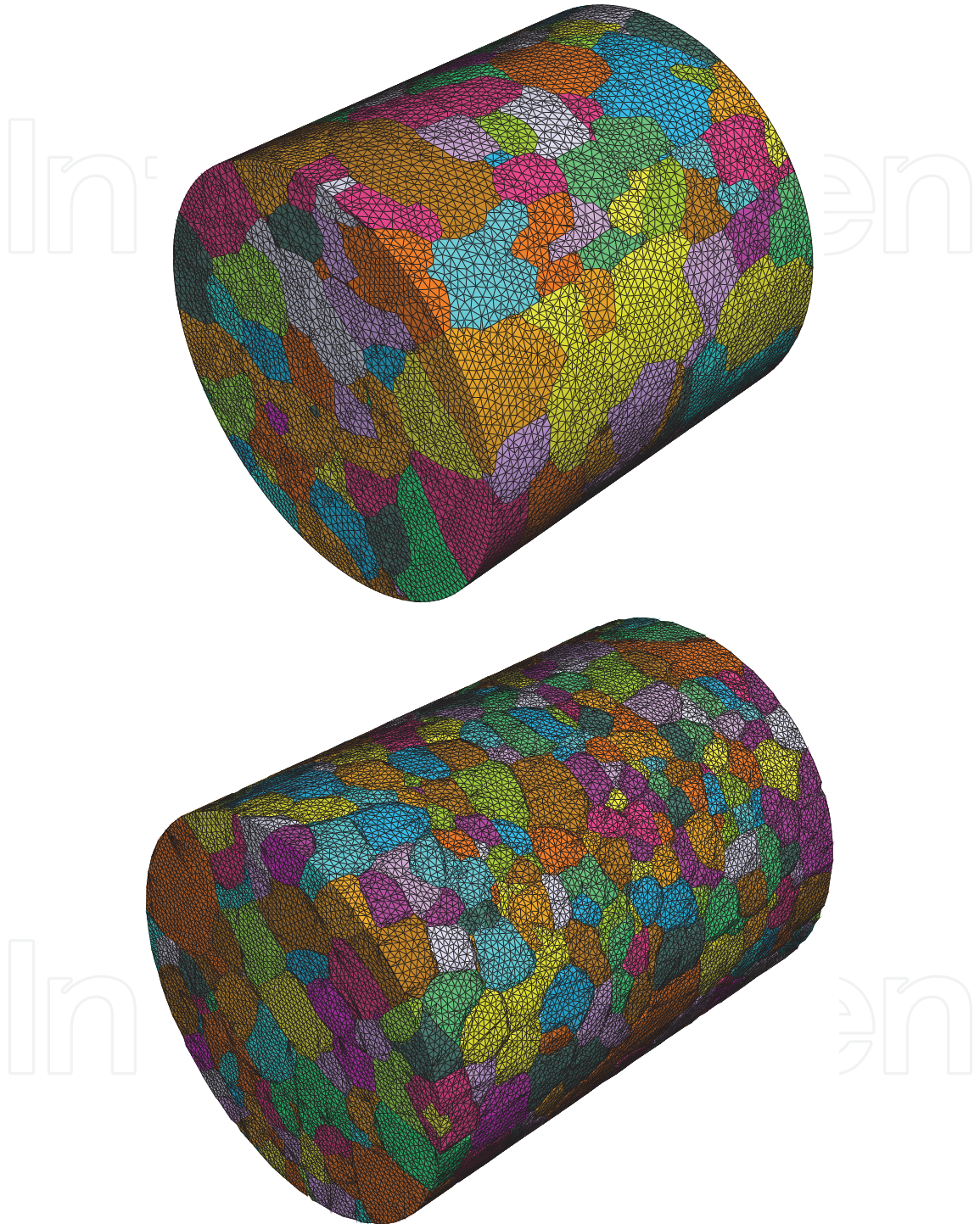
Fig. 11. A FE model of the 400\ \mu\text{m} diameter stainless steel wire. Top: wire from the first experimental series, 362 grains. Bottom: wire from the second experimental series, 1334 grains.
