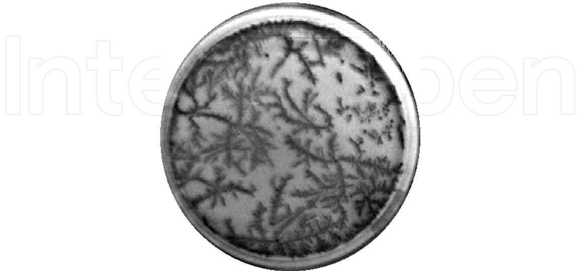
Fig. 8. DLA fractals in a PEO-NH 4 I membrane
