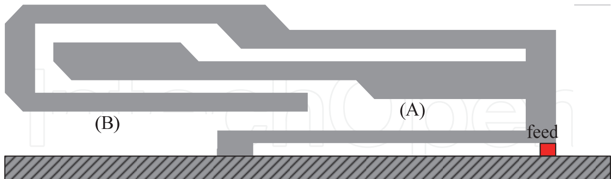
Fig. 5. A dual band inverted-F main resonator.
