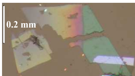
Fig. 2. Image under the optical microscope of \alpha -TPB crystals grown by the vapour transport method. It was taken with polarizer and analyser parallel to each other and to a crystal principal axis. Coloured fringes are interference fringes in regions of different thickness.
