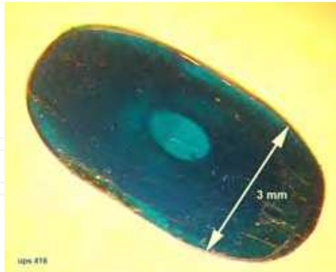
Fig. 6. Global view of a sample cleaved perpendicularly to its growth axis, the « a » axis. The sample composition was \text{CuGe}_{0.915}\text{Si}_{0.085}\text{O}_3 and it was grown at the rate 0.75-1.3 mm/h.
