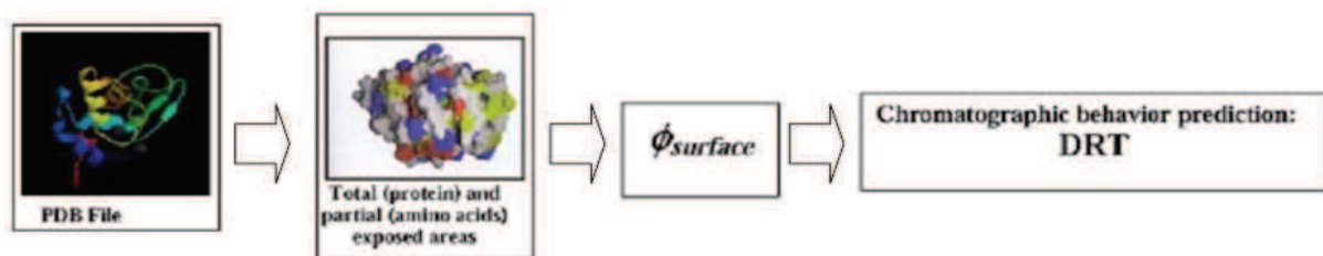
Fig. 5. Methodology for predicting protein retention time in HIC based on surface hydrophobicity. Using a PDB file as input to the program GRASP, the total and partial accessible areas of the exposed amino acids is determined. Using an amino acid hydrophobicity scale and equation (12), the average surface hydrophobicity can be obtained. Then, through simple mathematical correlations the DRT of the protein can be estimated.
