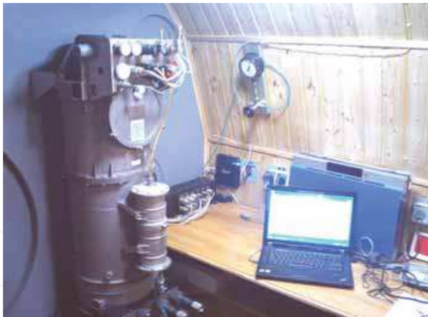
Fig. 16. Electrical trainer of the OGS-2 system based on the Electron-VM standard system.
