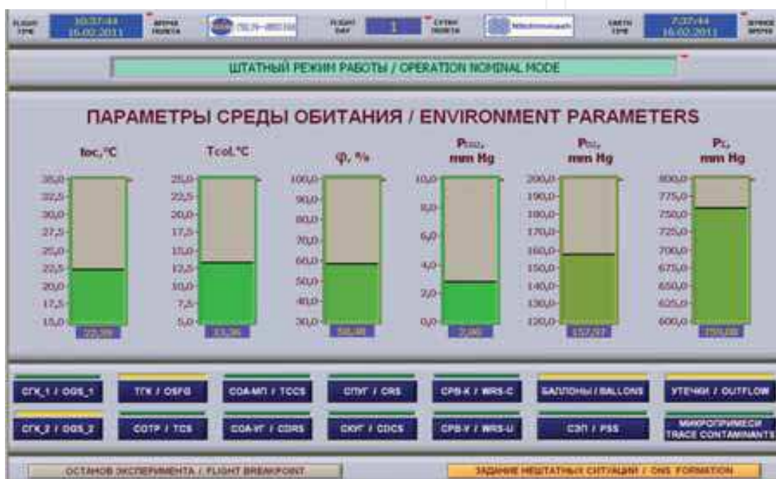
Fig. 7. Control panel of the 'PMM atmosphere' simulation model, where: t_{oc} , °C, T_{col} , °C, \phi , %, p_{CO_2} , mm of Hg, p_{O_2} , mm of Hg, p_{\Sigma} , mm of Hg = controllable parameter values.
