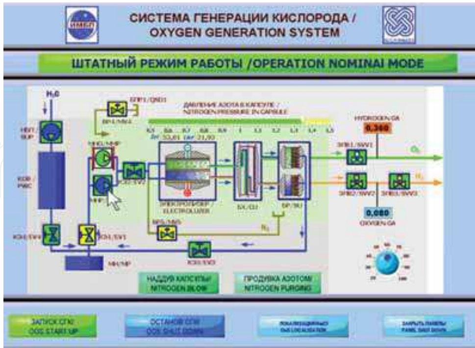
Fig. 11. Front panel of the ‘OGS’ virtual simulator subroutine in ‘OPERATION NOMINAL MODE’ (НБП/SUP=supply unit pump; КОВ/PWC=pre-purification water container; КЭИ/EVI=electromagnetic valve; МНО/MMP and МНР/RMP=main micro-pump and reserve micro-pump; БХ/СU=cooling unit; БР/SU=separator unit; GA=gas analyzer).
