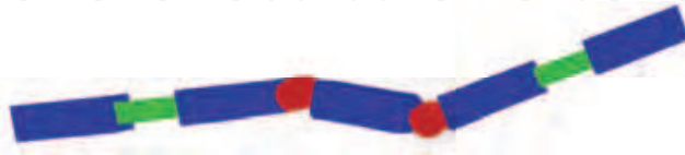
Fig. 2. Example of an articulated object. Links (rigid bodies) are shown in blue. Revolute joints are represented by red cylinders, and prismatic joints are illustrated as green boxes. Joint types are only marked for illustrative purposes but not in the experiments.
