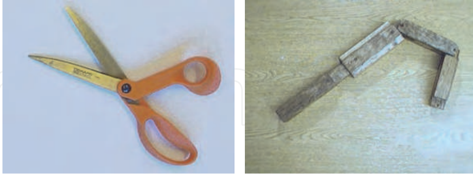
Fig. 1. Two examples of kinematic structures: scissors with a single revolute joint and a wooden toy with a prismatic joint and two revolute joints.
