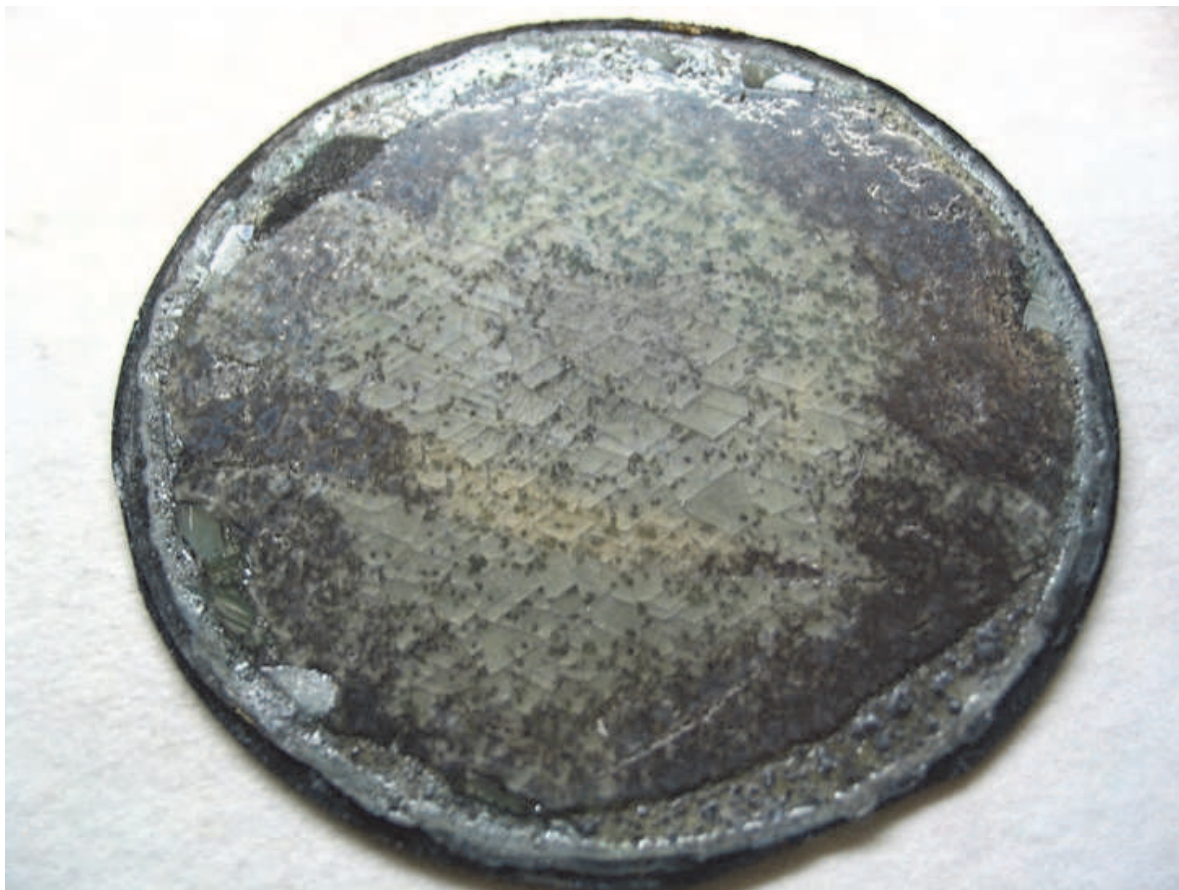
Fig. 11. 2in AlN seed grown on 60 mm micropipe-free SiC substrate.
